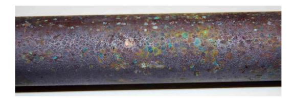
Typically samples of failed pipe and foam insulation associated with the leak failure are sent to LPD Lab Services for investigation. The pipework is assessed by optical microscopy as well as SEM/EDX determining the root cause and corrosion mechanism. Additionally the foam insulation is soaked in water and the resulting solution is analysed for pH, to check if it is acidic, and for the presence of aggressive species by lon Chromatography (IC).
