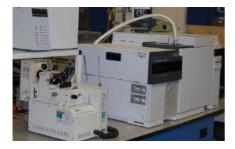
This hybrid technique links a pyrolyser to a GC-MS allowing direct sample preparation and injection into the GC-MS. The process, put simply will break apart large, complex organic molecules into smaller,
