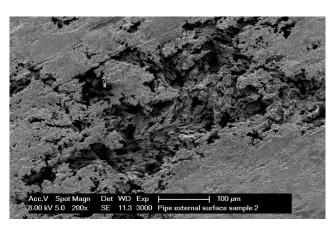
pitting, or galvanic attack behaviour, is to use Potentiostat Electrochemical Testing, which is an excellent way to assess susceptibility to corrosion mechanisms on manufactured parts in an accelerated way.
