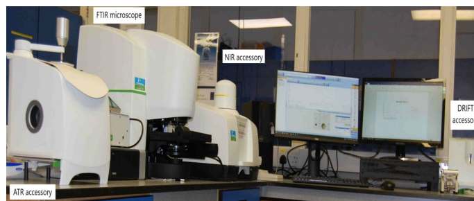
Perkin Elmer Frontier FTIR with Spotlight microscope and accessories
