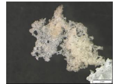
Packing material – Polyurethane prepolymer - Not fully cured - Not a source of inorganic debris
